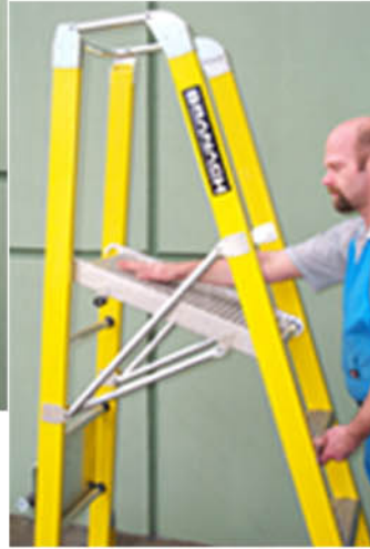
Push platform and allow ladder to move forward
