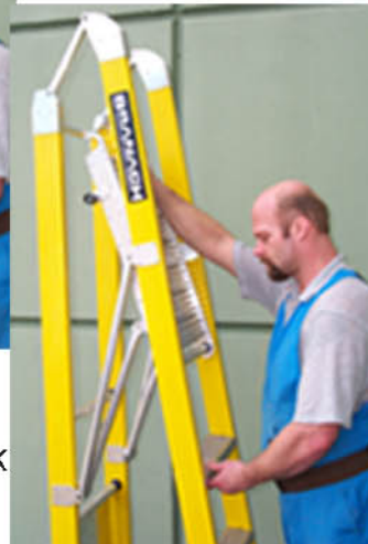
Pull platform fully forward allowing sections to close
